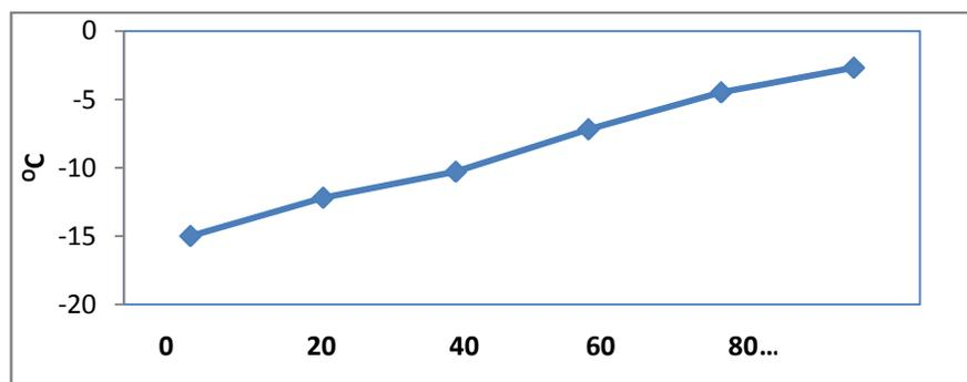
Figure 3: Plot of pour point against percentage concentration of biodiesel
