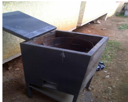
Plate 1: A locally fabricated reactor used for biochar production
