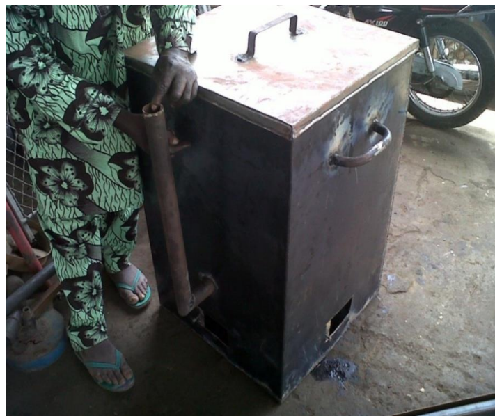
Plate 1: Pictorial view of the fabricated charcoal-fired kiln
